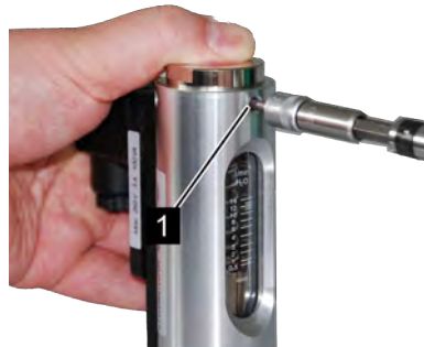
Fig. 57: Tighten hex socket screws
