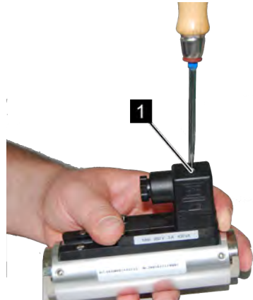
Fig. 59: Loosen female socket
