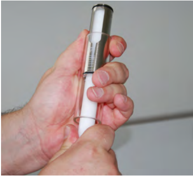
Fig. 41: Remove slot nozzle
