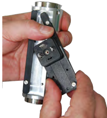
Fig. 63: Rotate guide rail to the side
