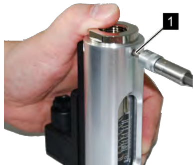
Fig. 53: Secure the process connection
