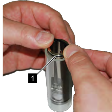
Fig. 47: Centering the slot nozzle
