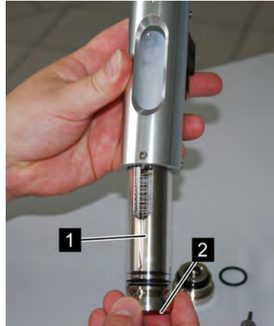
Fig. 40: Remove the inner section
