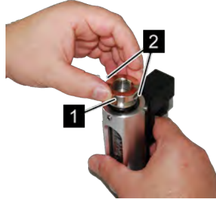
Fig. 56: Position the outlet process connection
