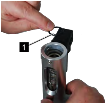
Fig. 55: Slot nozzle buffer
