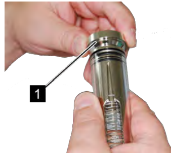
Fig. 50: Process connection (Inlet)
