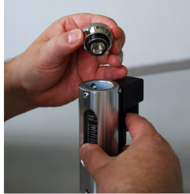
Fig. 37: Remove the process connection (outlet)
