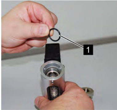
Fig. 38: Slot nozzle buffer O-ring
