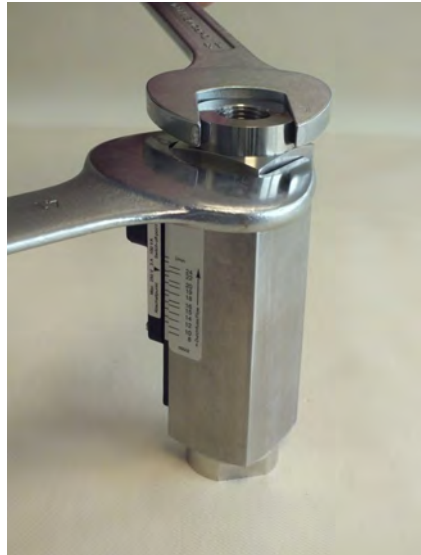
Fig. 43: Loosen process connection (outlet)
