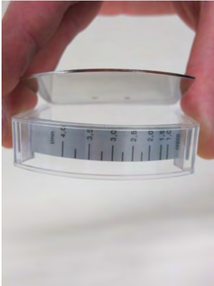
Fig. 40: Removal of display cover plate from housing
