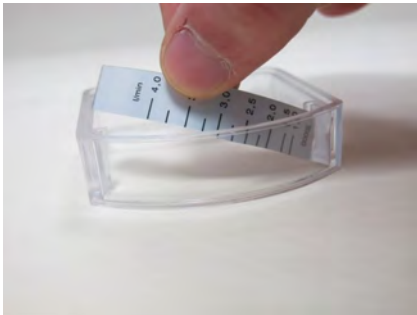
Fig. 41: Removal of the scale support
