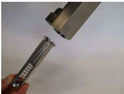
Fig. 55: Insert inner parts
