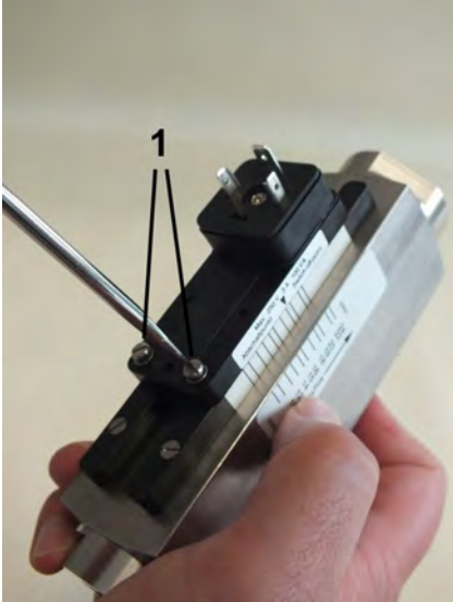
Fig. 35: Loosen the set screws
