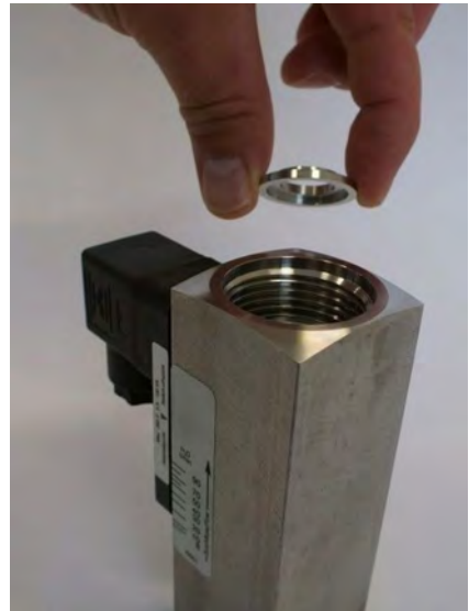
Fig. 45: Remove the centering disc (outlet)
