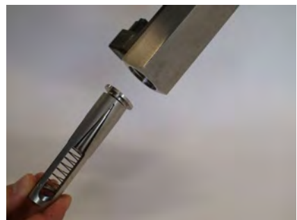
Fig. 46: Remove inner parts
