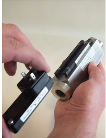
Fig. 69: Remove switch contact
