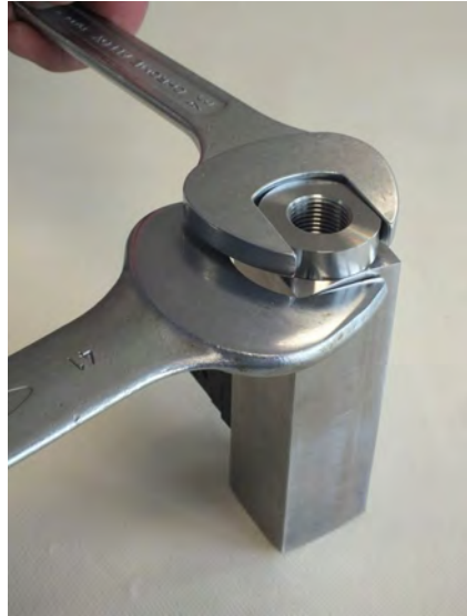
Fig. 48: Loosen process connection (inlet)
