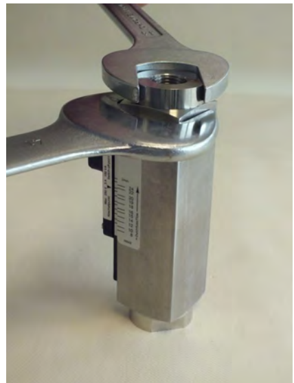
Fig. 36: Loosen process connection (outlet)
