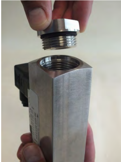
Fig. 50: Insert process connection (outlet)
