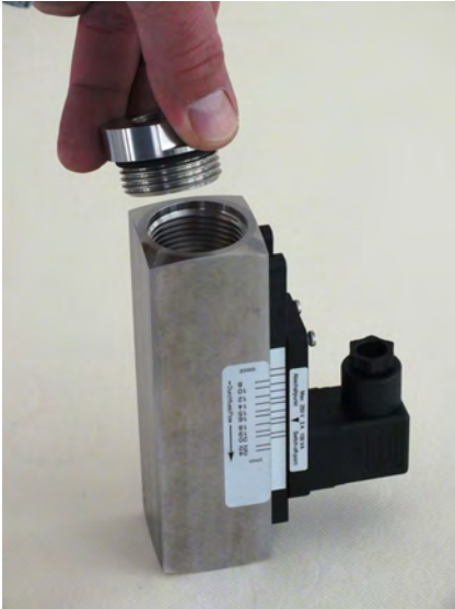
Fig. 42: Remove the process connection (inlet)
