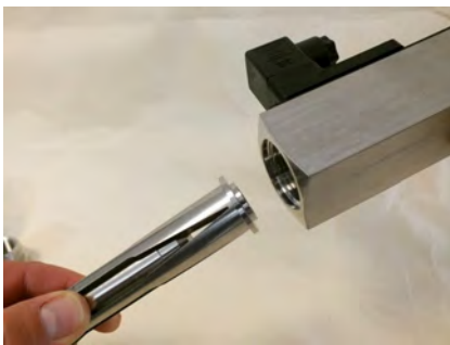
Fig. 48: Insert inner parts
