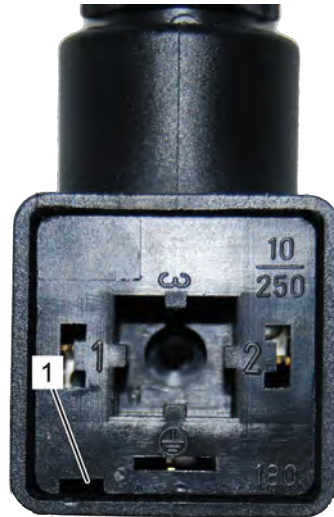
Fig. 24: Loosen inner section
