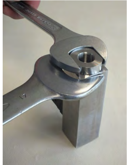
Fig. 46: Tighten process connection (inlet)
