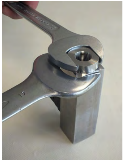
Fig. 41: Loosen process connection (inlet)
