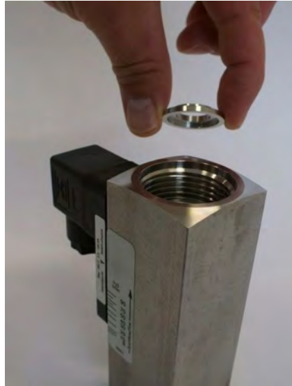
Fig. 38: Remove the centering disc (outlet)
