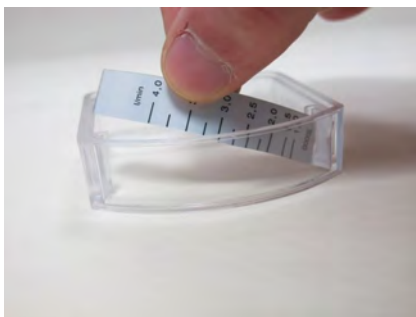
Fig. 41: Removal of the scale support
