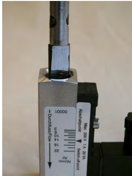
Fig. 43: Seat threaded ring (inlet)
