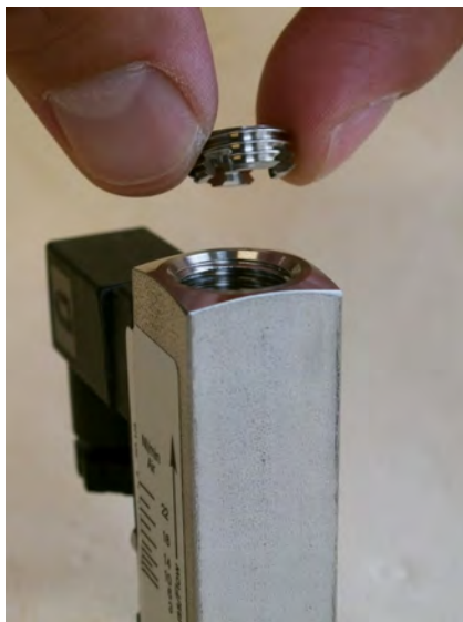
Fig. 36: Remove threaded ring (outlet)
