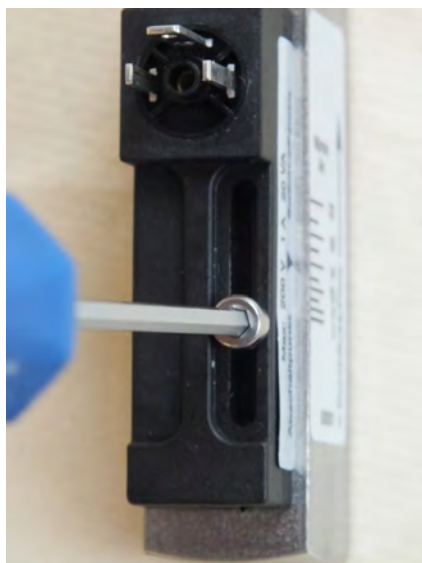
Fig. 31: Loosen set screw
