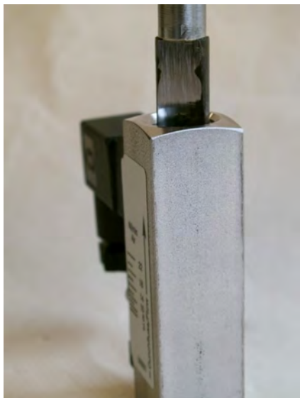
Fig. 35: Loosen threaded ring (outlet)
