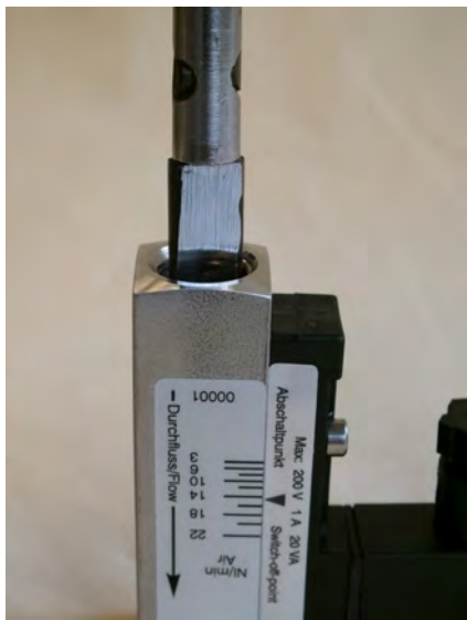
Fig. 40: Loosen threaded ring (inlet)
