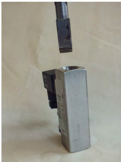
Fig. 34: Insert threaded ring insertion tool (outlet)
