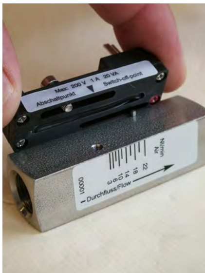
Fig. 52: Remove switch contact
