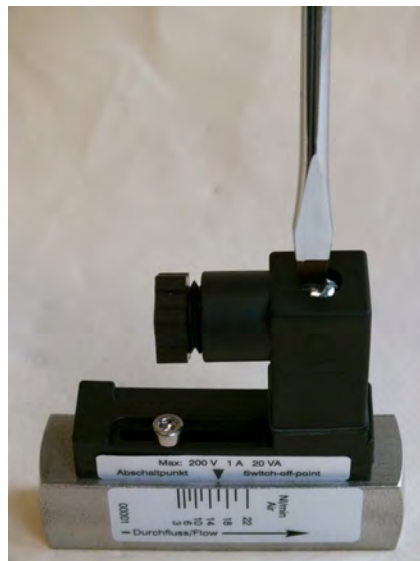
Fig. 49: Loosen female socket
