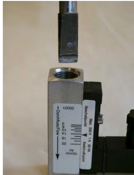
Fig. 39: Insert threaded ring insertion tool (inlet)
