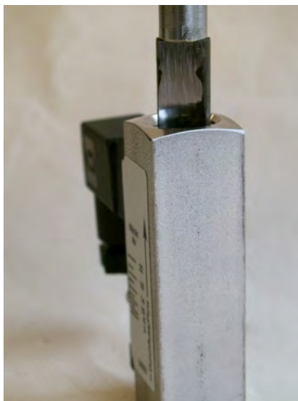
Fig. 47: Seat threaded ring (outlet)
