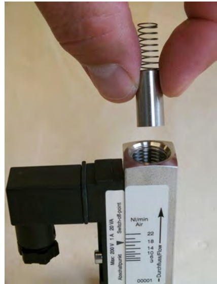
Fig. 45: Insert inner parts
