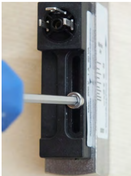
Fig. 51: Loosen set screw
