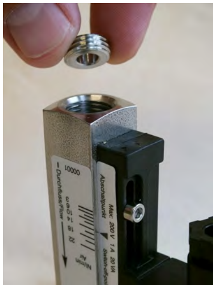
Fig. 41: Remove threaded ring (inlet)
