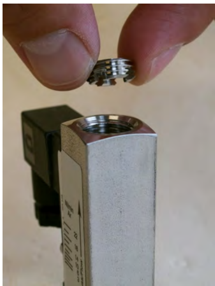
Fig. 46: Insert threaded ring (outlet)
