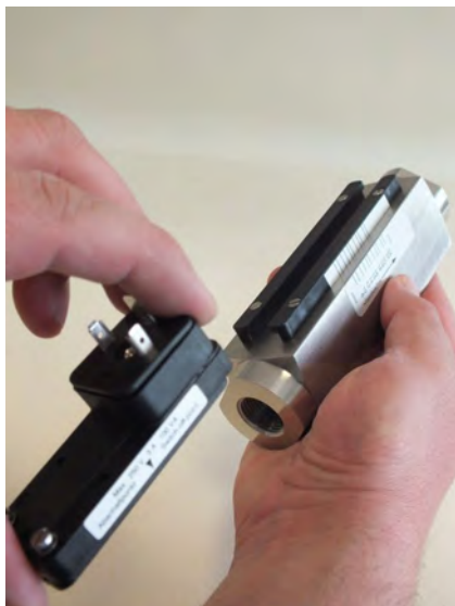
Fig. 77: Remove switch contact
