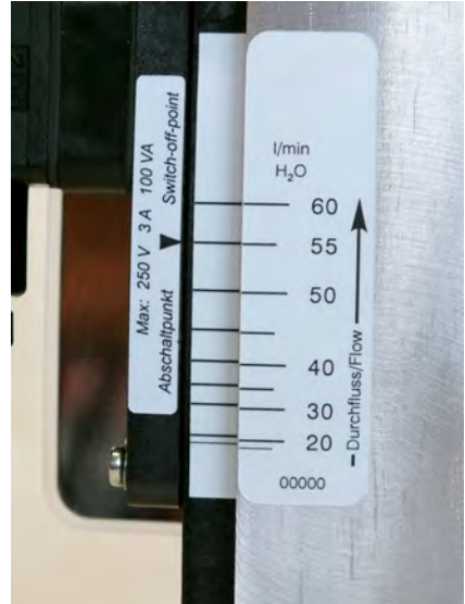
Fig. 4: Switch point adjustment scale
