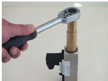
Fig. 46: Loosen threaded ring (outlet)
