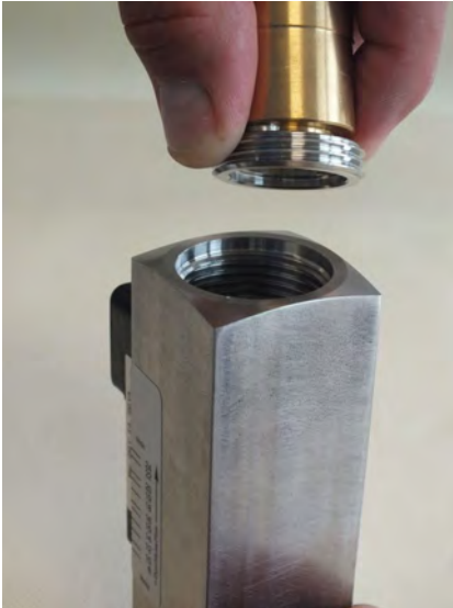
Fig. 47: Remove threaded ring (outlet)
