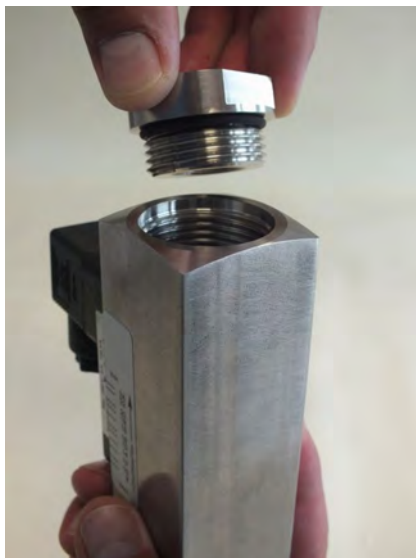
Fig. 65: Insert process connection (outlet)
