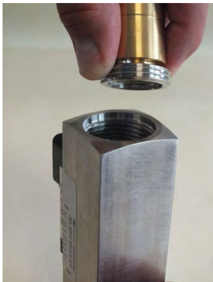
Fig. 63: Insert threaded ring (outlet)
