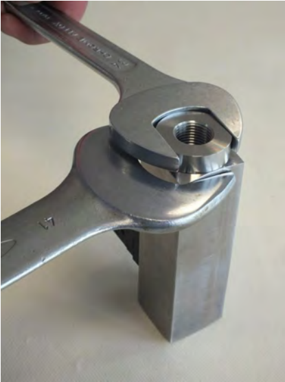
Fig. 50: Loosen process connection (inlet)
