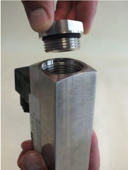
Fig. 44: Remove the process connection (outlet)
