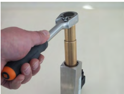
Fig. 53: Loosen threaded ring (inlet)
