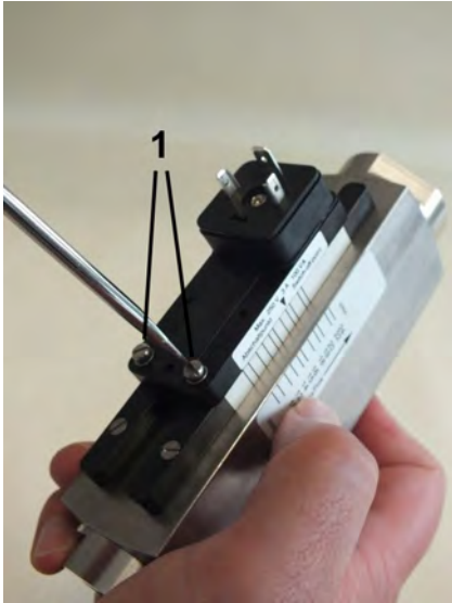
Fig. 75: Loosen set screws
