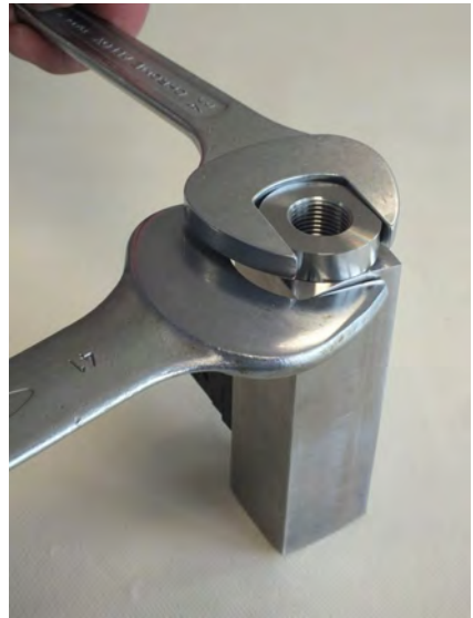
Fig. 60: Tighten process connection (inlet)
