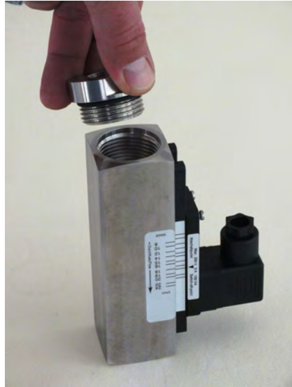
Fig. 51: Remove the process connection (inlet)
