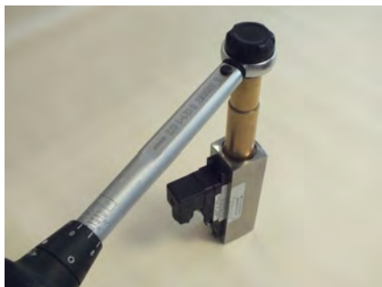
Fig. 64: Seat threaded ring (outlet)
