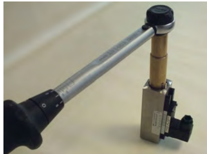
Fig. 58: Seat threaded ring (inlet)
