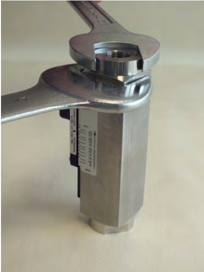
Fig. 66: Tighten process connection (outlet)
