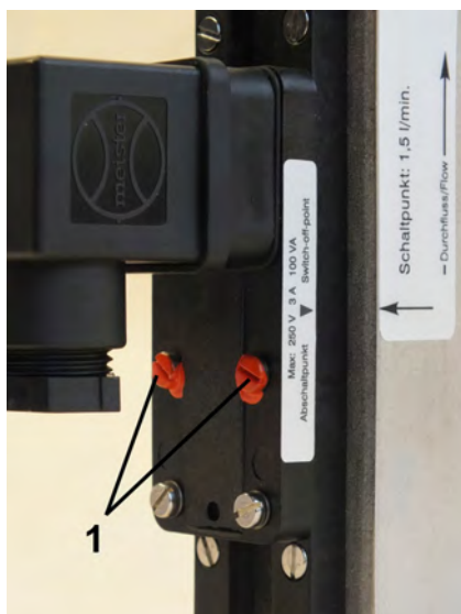
Fig. 33: Locked switch point
