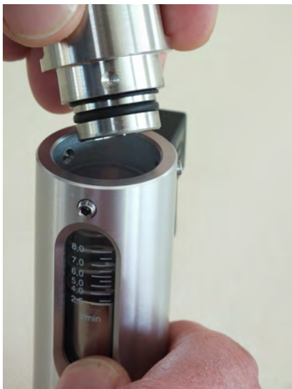
Fig. 36: Remove the process connection (outlet)
