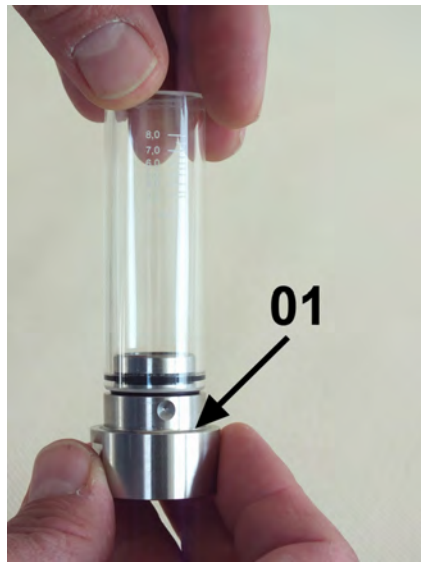
Fig. 44: Process connection (inlet) in sight glass
