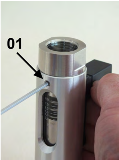
Fig. 51: Tighten hex socket screws
