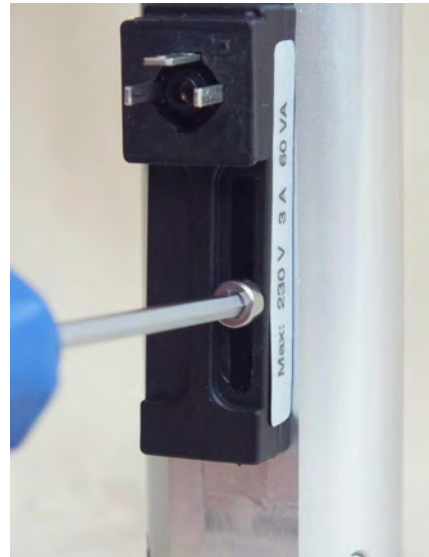
Fig. 32: Loosen set screw
