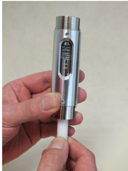
Fig. 52: Check for ease of movement
