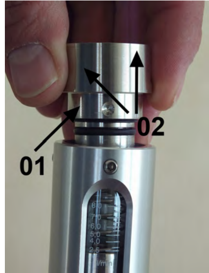
Fig. 50: Position process connection (outlet) in device housing
