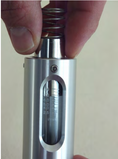
Fig. 49: Insert float and inner parts
