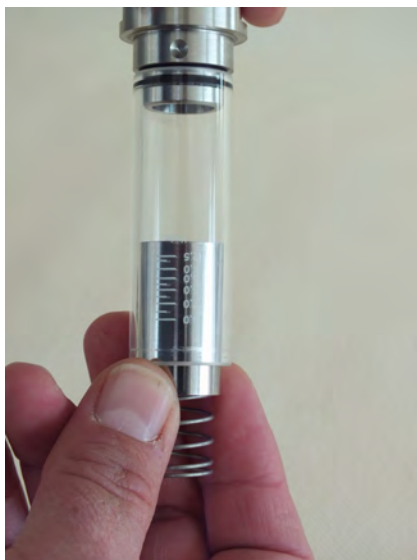
Fig. 39: Remove float, magnets and spring
