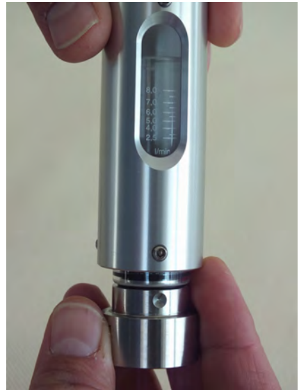
Fig. 46: Insert the process connection into the device housing
