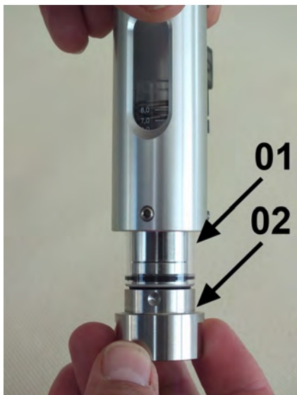
Fig. 38: Remove the inner section
