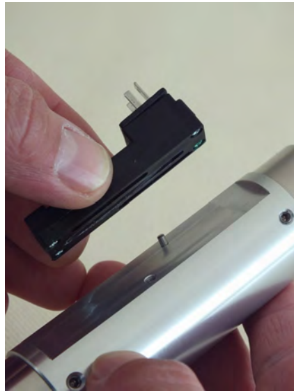
Fig. 56: Remove switch housing
