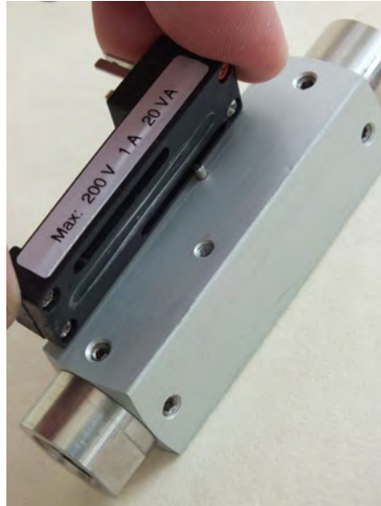
Fig. 56: Remove switch housing
