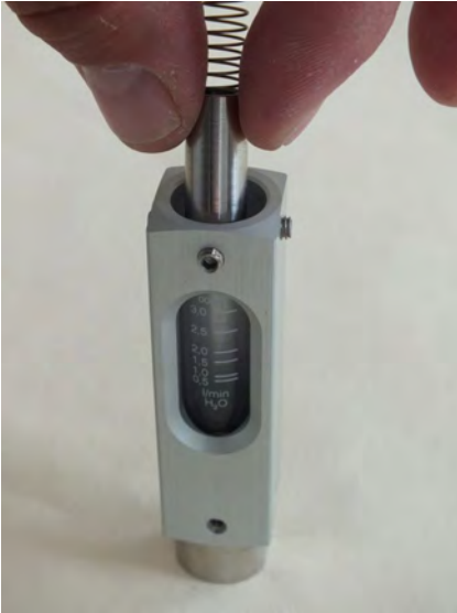
Fig. 49: Insert float and inner parts
