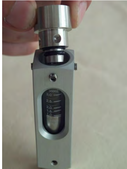
Fig. 36: Remove the process connection (outlet)
