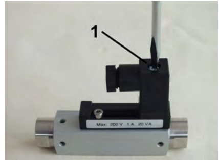
Fig. 53: Loosen female socket
