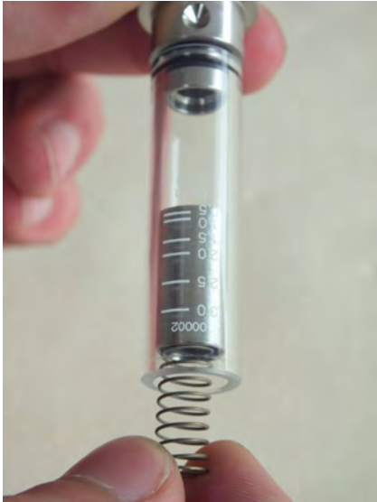
Fig. 39: Remove float, magnets and spring
