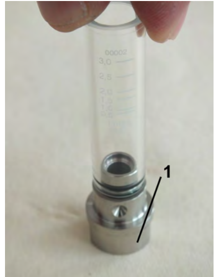
Fig. 44: Process connection (inlet) in sight glass
