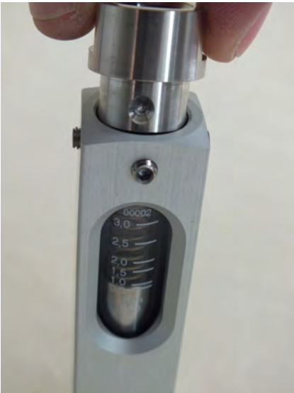
Fig. 51: Tighten hex socket screws
