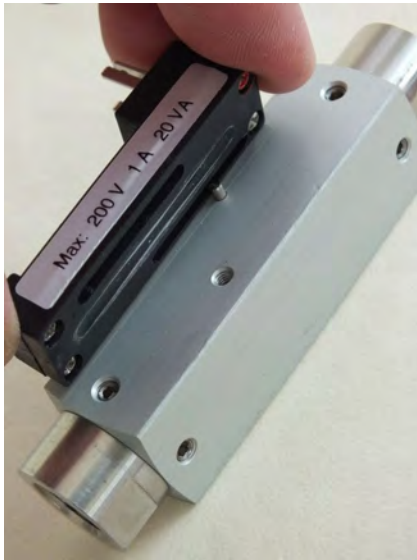
Fig. 55: Remove switch contact
