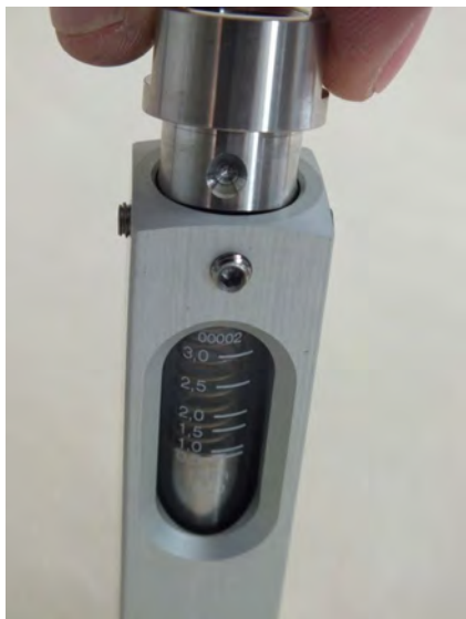
Fig. 49: Position the process connection (outlet)
