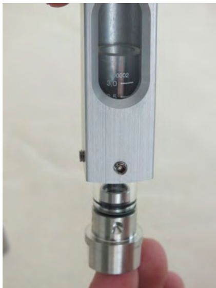
Fig. 45: Insert process connection into device housing
