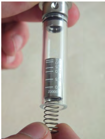
Fig. 38: Remove float and spring
