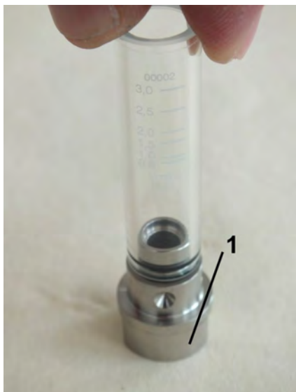
Fig. 43: Process connection (inlet) and sight glass
