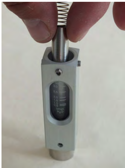
Fig. 48: Insert the inner parts
