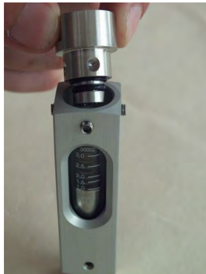
Fig. 35: Remove the process connection (outlet)
