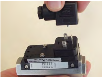
Fig. 55: Remove female socket
