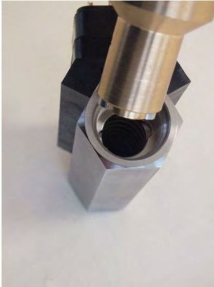
Fig. 36: Insert threaded ring insertion tool (outlet)
