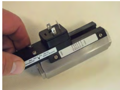
Fig. 57: Remove switch contact from guide rails
