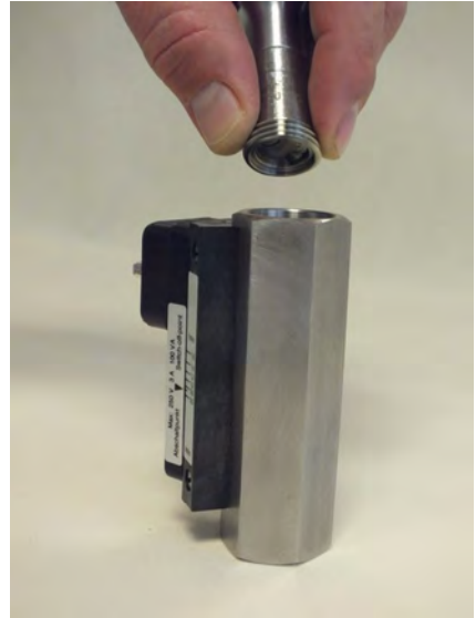
Fig. 38: Remove threaded ring (outlet)
