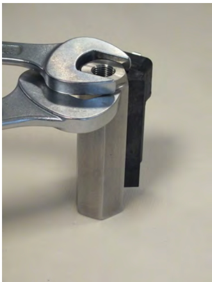
Fig. 34: Loosen process connection (outlet)
