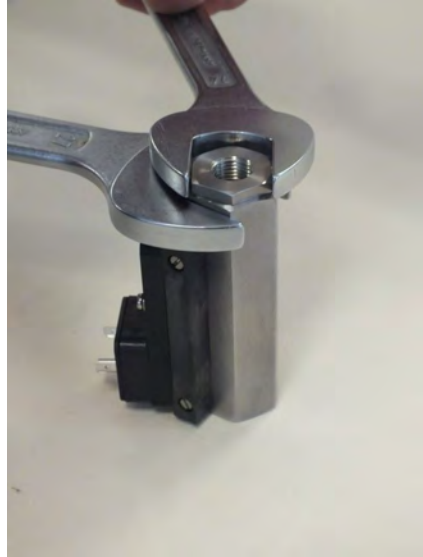
Fig. 41: Loosen process connection (inlet)
