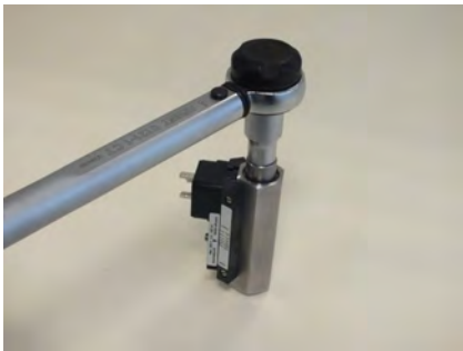
Fig. 37: Loosen threaded ring (outlet)
