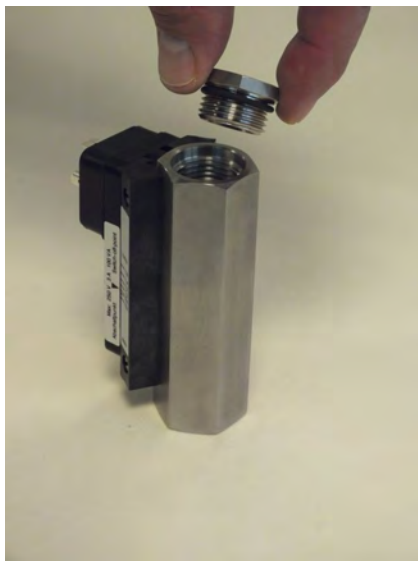
Fig. 35: Remove the process connection (outlet)
