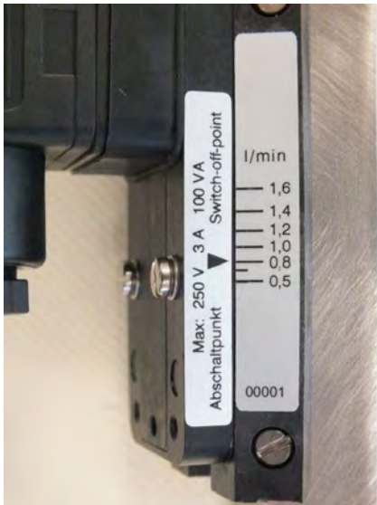
Fig. 33: Reading-off the switch point value
