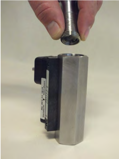
Fig. 49: Insert threaded ring (outlet)
