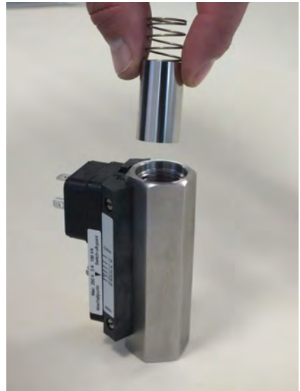
Fig. 48: Insert inner parts
