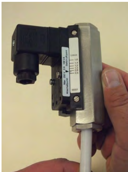
Fig. 53: Check for smooth operation
