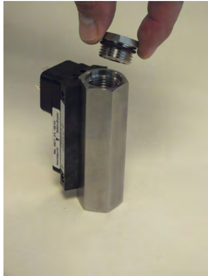
Fig. 51: Insert process connection (outlet)
