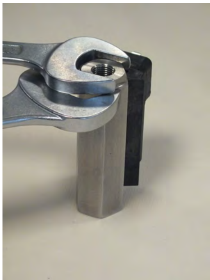
Fig. 52: Tighten process connection (outlet)
