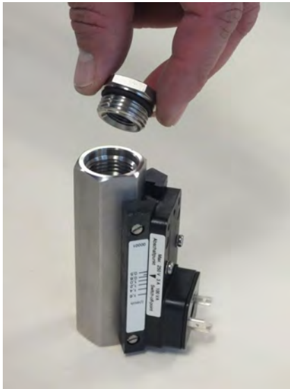
Fig. 42: Remove the process connection (inlet)
