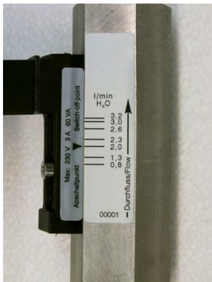
Fig. 34: Reading-off the switch point value
