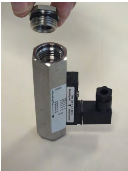
Fig. 46: Insert process connection (inlet)
