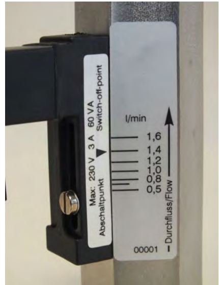
Fig. 4: Switch point adjustment scale DKM-2
