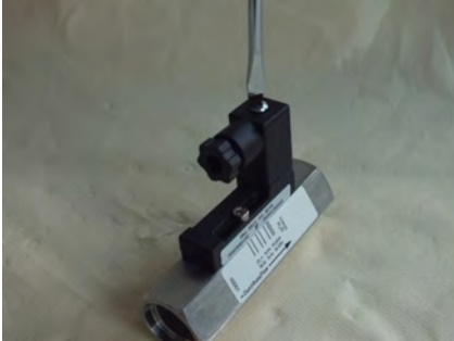
Fig. 55: Loosen female socket
