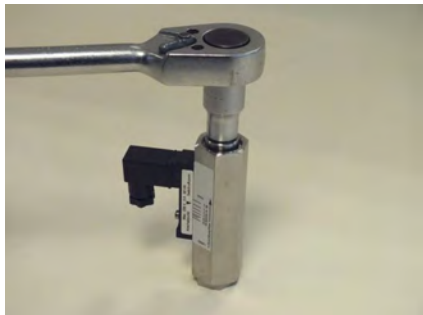
Fig. 51: Seat threaded ring (outlet)
