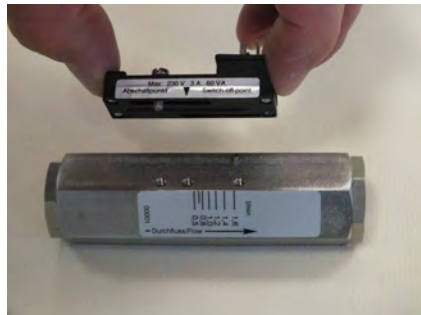
Fig. 58: Remove switch contact
