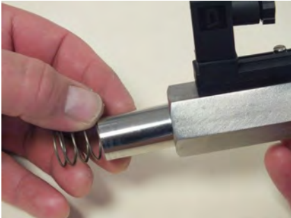
Fig. 40: Remove inner parts
