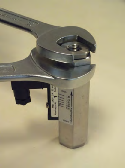
Fig. 35: Loosen process connection (outlet)
