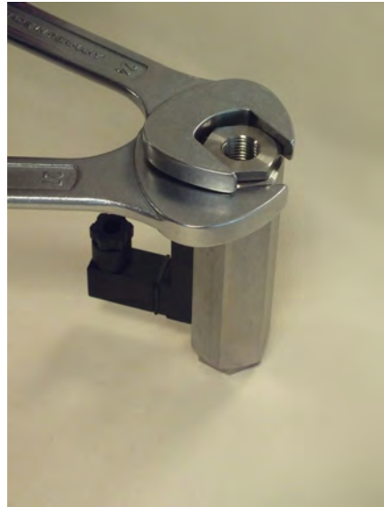
Fig. 42: Loosen process connection (inlet)
