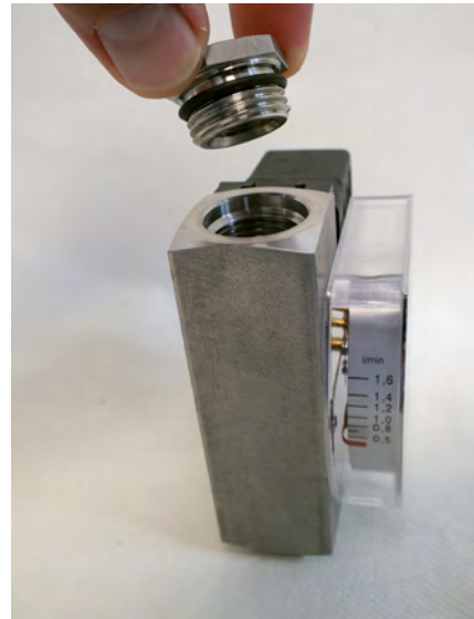
Fig. 44: Remove the process connection (outlet)
