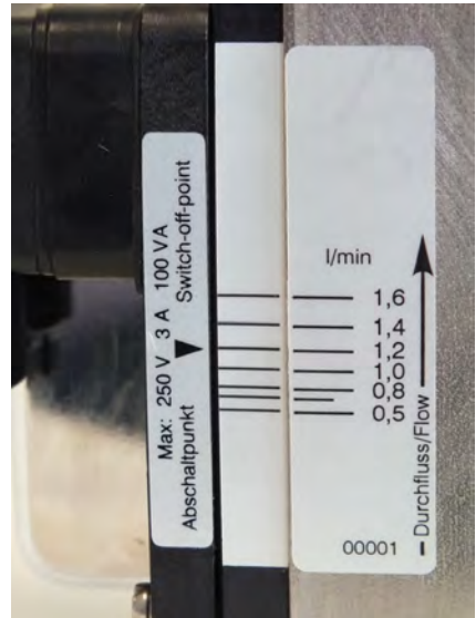
Fig. 4: Switchpoint adjustment scale DKM/A-2 30x70
