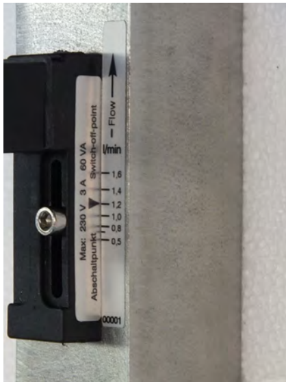
Fig. 35: Reading-off the flow value
