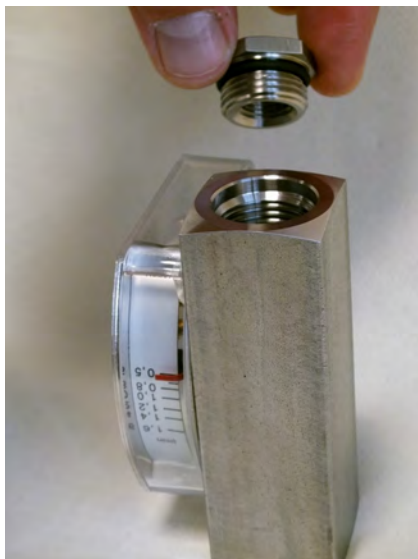
Fig. 50: Remove process connection (inlet)
