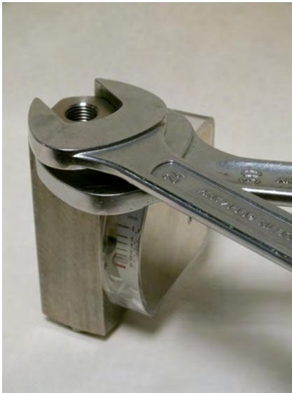
Fig. 42: Loosen process connection (outlet)
