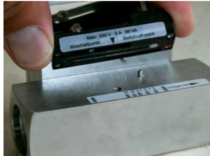
Fig. 70: Remove switch housing
