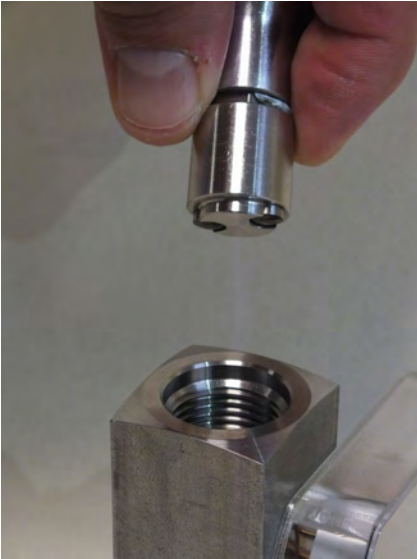
Fig. 44: Insert threaded ring insertion tool (outlet)
