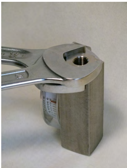
Fig. 49: Loosen process connection (inlet)
