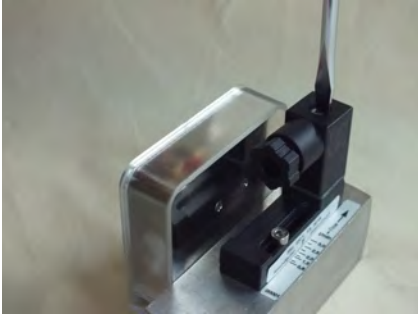
Fig. 67: Loosen female socket
