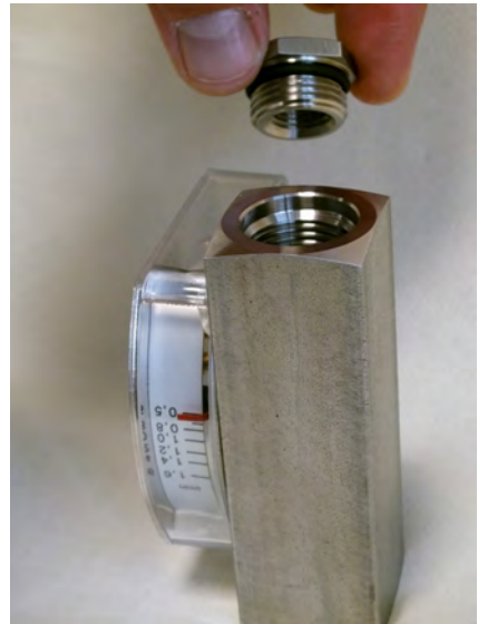
Fig. 53: Insert process connection (inlet)
