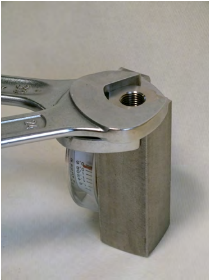
Fig. 54: Tighten process connection (inlet)
