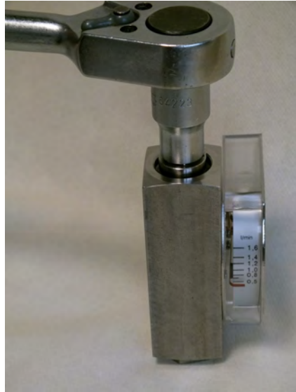
Fig. 45: Loosen threaded ring (outlet)
