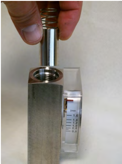
Fig. 56: Insert inner parts
