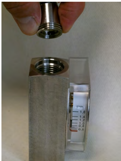
Fig. 46: Remove threaded ring (outlet)
