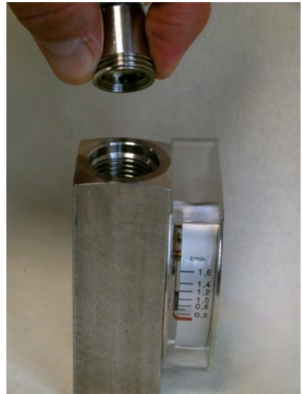
Fig. 57: Insert threaded ring (outlet)
