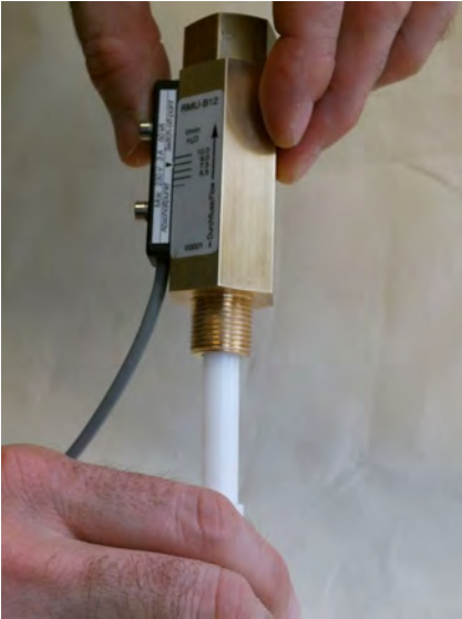
Fig. 36: Check for smooth operation
