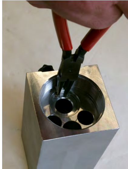
Fig. 43: Secure snap ring in groove
