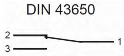
Fig. 15: Switch position under no-flow condition
