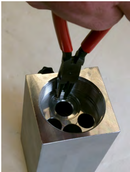
Fig. 36: Loosen snap ring (inlet)
