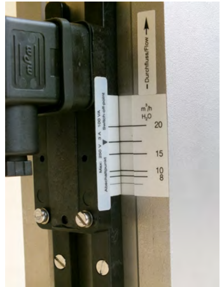
Fig. 4: Switch point adjustment scale (example)
