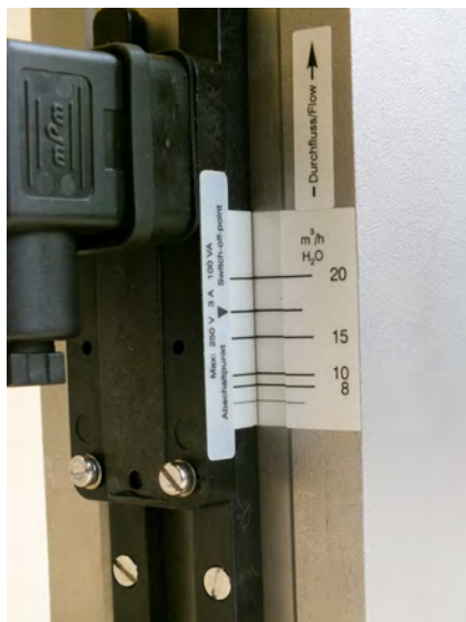
Fig. 35: Reading-off the switch point (example)
