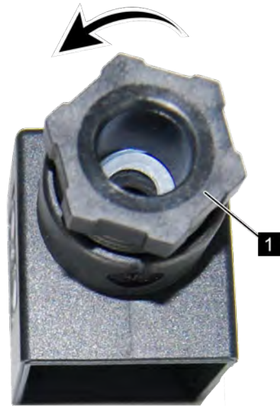
Fig. 25: Loosen the screw connection
