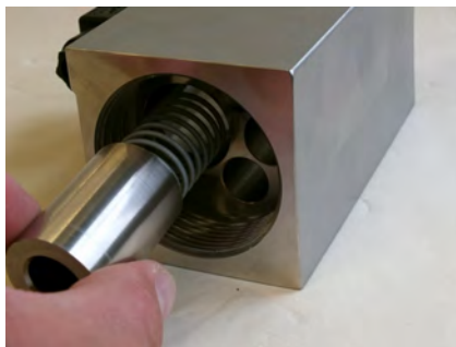
Fig. 38: Remove inner parts
