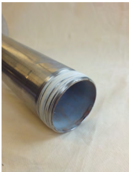
Fig. 10: Pipe connection with sealing thread
