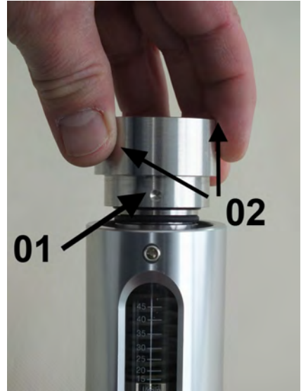
Fig. 51: Position process connection (outlet) in device housing
