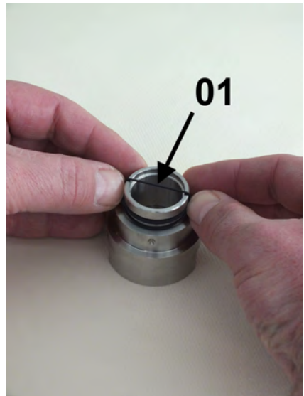
Fig. 42: O-ring (Glass buffer)
