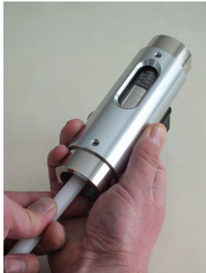
Fig. 53: Check for free movement
