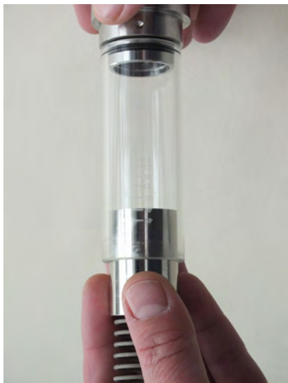
Fig. 40: Remove float, magnets and spring
