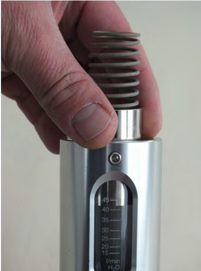
Fig. 50: Insert float and inner parts
