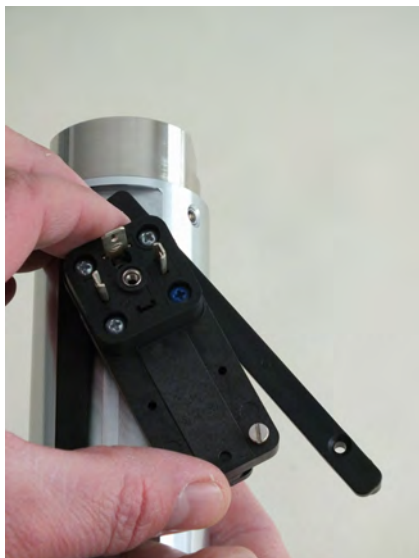
Fig. 58: Rotate guide rail to the side
