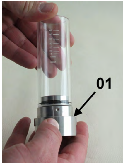
Fig. 45: Process connection (inlet) in sight glass
