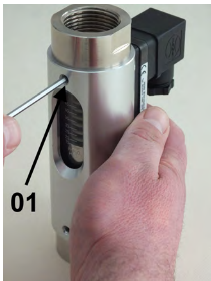
Fig. 37: Remove the process connection (outlet)
