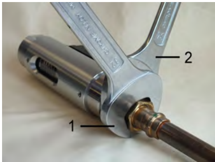
Fig. 11: Screw in the device
