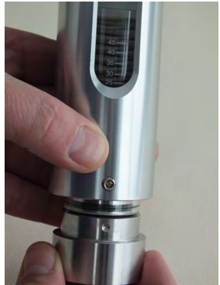
Fig. 47: Insert the process connection into the device housing
