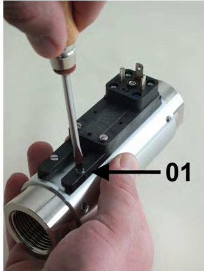
Fig. 57: Release the guide rail
