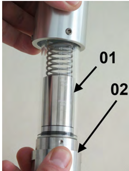
Fig. 39: Remove inner section
