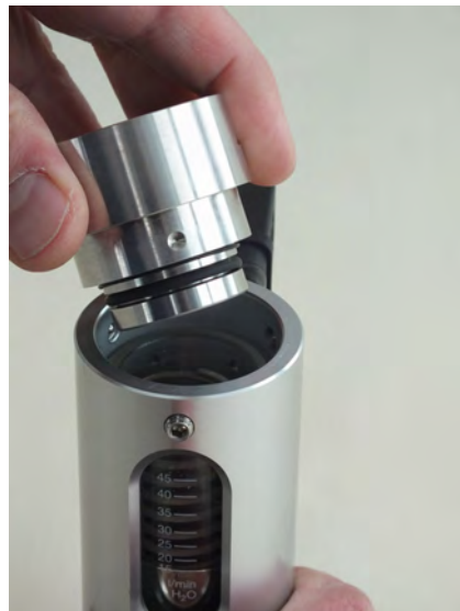
Fig. 37: Remove the process connection (outlet)
