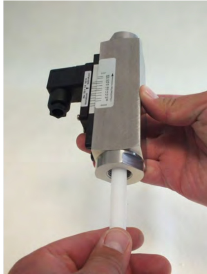
Fig. 67: Check for smooth operation
